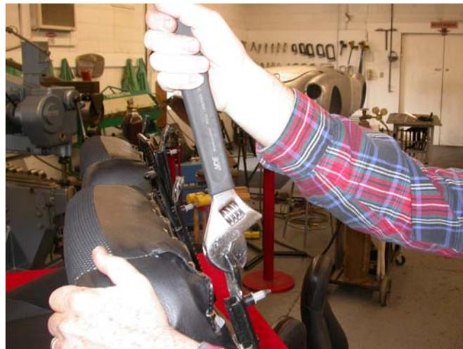
Once you've done the front parts of the rails, flip the seats over and repeat on the rear part of the rails.
